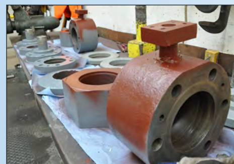
Above, left: Hardware parts used for attaching a turbine headgate to its pinning beam are cleaned and repainted to prevent rust development when in use. Above, right: Colbey Soule, powerplant mechanic, and Ben Muzzey, utility worker, install new roller chain on a turbine headgate at McNary Lock and Dam.
