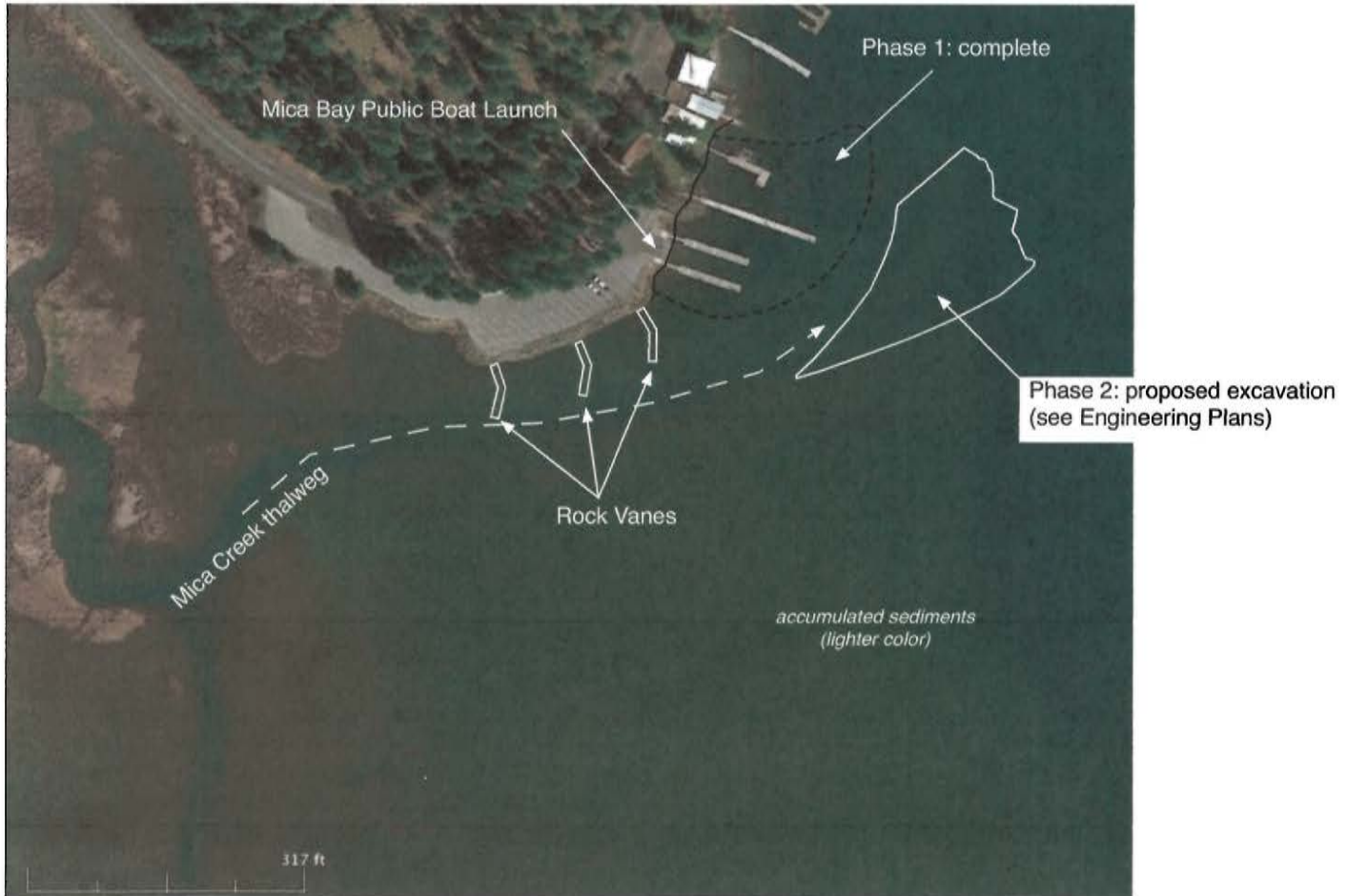
overall view of project area: locations approximate (see Engineering Plans for actual locations and detail)
