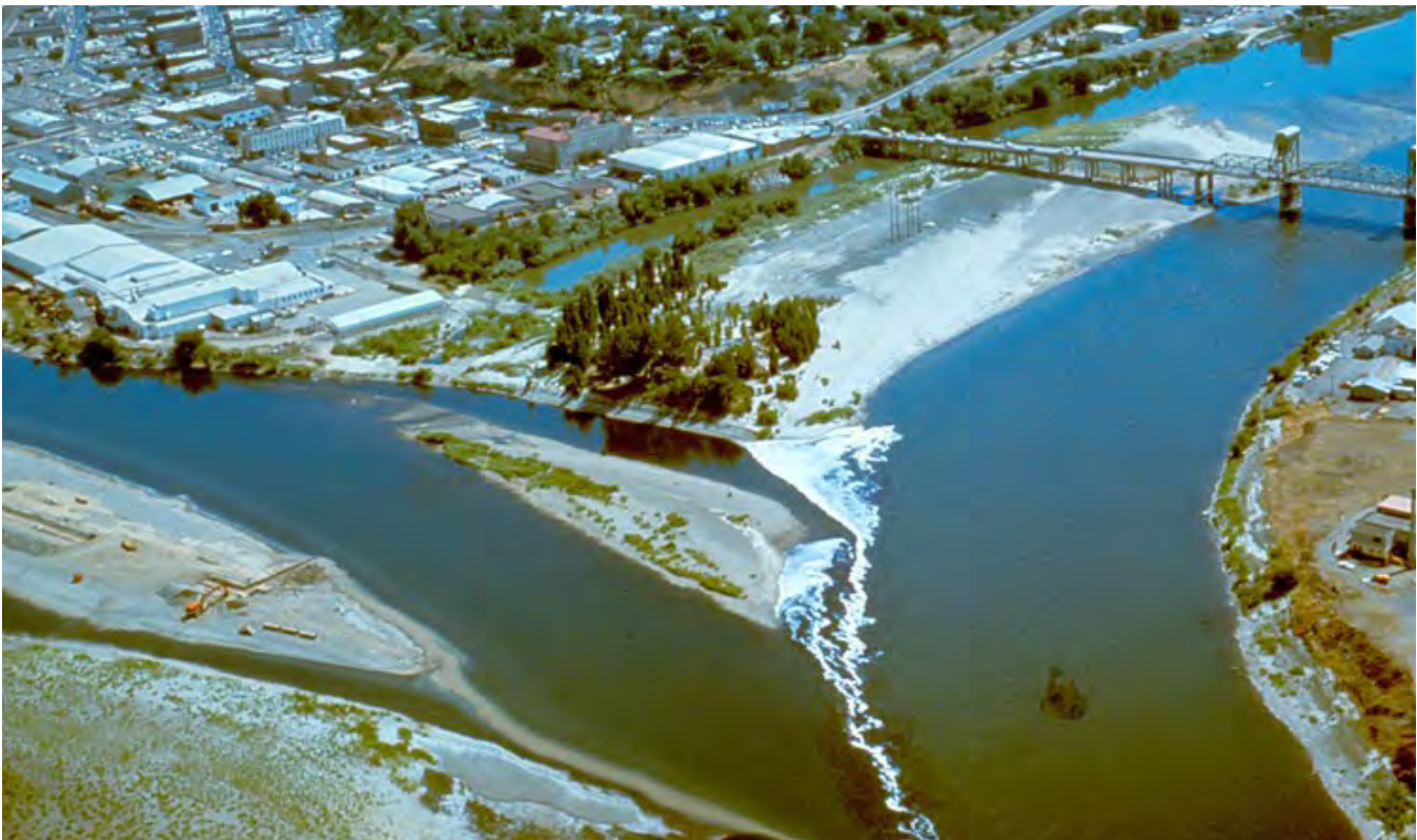
Figure 6-3. Sediment Deposition at the Confluence of the Clearwater and Snake Rivers
