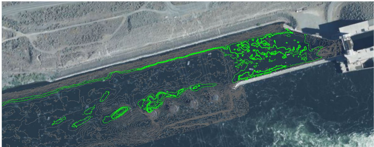
Figure 3. Shoaling at Ice Harbor navigation lock approach. Areas less than 16 ft deep at Minimum Operating Pool (MOP) are in green.
