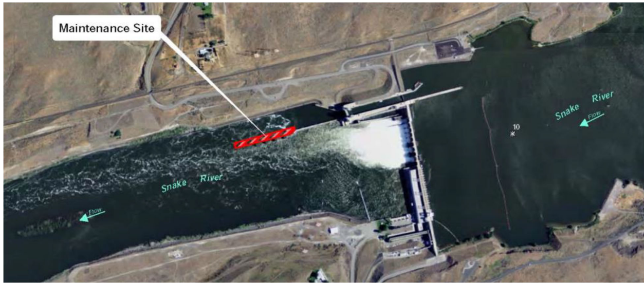
Figure 2. Dredging location at Ice Harbor navigation lock approach.
