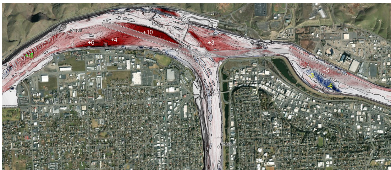
Figure 7. Sediment Deposition Difference Between 2021 and 2011
