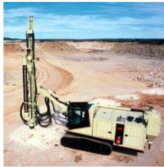
They said it couldn't be done... hey were wrong. The new ECM-720 crawler drill delivers a perfect balance of productivity and cost efficiency. Hole straightness, faster penetration rates, long accessory life, and increased profitability are just a few of the results you can expect with the ECM-720.
