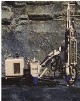
The ECM-590 is a self-contained, cableless hydraulic crawler drill capable of drilling up to 4 in. (102 mm) holes. It is available in either a YH70 drifter and rod rack configuration for smaller hole work, or with a YH80 and rod changer for higher production requirements. An extended guide option for 20 ft. (6.1 m) starter steel is available.
