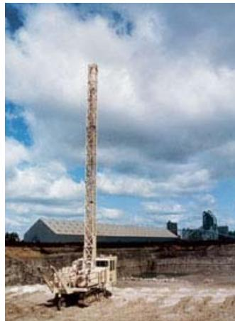
The DM25SP is a crawler-mounted rotary table drill rig designed for single-pass blasthole drilling to depths of up to 50 ft. (15.2 m) and diameters of 3-1/2 to 6-3/4 in. (89 to 171 mm). This drill is capable of rotary drilling with 25,000 lb. (11,340 kg) of bit load at 0-200 rpm. The DM25SP can also be used with downhole drills when equipped with a high-pressure air compressor option.
