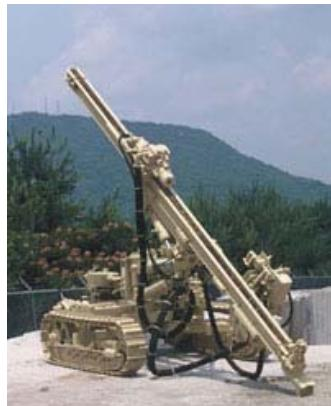
The LM100A is a small class pneumatic Crawlair<sup>?</sup>, capable of drilling 1-3/4" to 4- 1/2" (44 - 114 mm) diameter holes. It can be equipped with either of two drifters or a BRH rotary head for downhole drilling. The LM100A is ideal for applications in confined areas where hand-held tools are not enough, and is light enough to transport by helicopter. Like all Ingersoll-Rand crawler drills, the LM100A is "Abuse Resistant". It keeps coming back for more!
