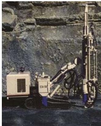
The ECM-590 is a self-contained, cableless hydraulic crawler drill capable of drilling up to 4 in. (102 mm) holes. It is available in either a YH70 drifter and rod rack configuration for smaller hole work, or with a YH80 and rod changer for higher production requirements. An extended guide option for 20 ft. (6.1 m) starter steel is available.
