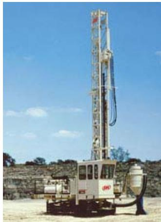
The DM30 is a hydraulic tophead drive, multi-pass, crawler-mounted drill rig designed for blastholes ranging from 5-1/8 to 6-3/4 in. (130 to 171 mm) in diameter. On-board depth capability is up to 150 ft. (45.7 m). For rotary drilling, the DM30 can assert a bit load force up to 30,000 lb. (13,608 kg) and rotation speeds of 0-130 RPM. This rig can also be used with downhole drills when equipped with a high-pressure air compressor option.
