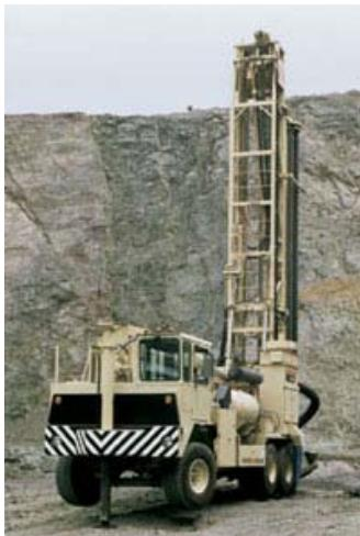
The T4BH is a truck-mounted, hydraulic tophead drive multi pass rotary drill specifically designed for production blast hole drilling to depths of 150 ft. (45.7 m) with a 25 ft. (7.6 m) drill pipe change. Nominal hole size is 5-1/8 to 7-7/8 in. (130 to 200 mm) for rotary or DHD drilling methods. Feed pressure generates a bit load force of up to 30,000 lb. (12,610 kg). An angle drilling option is available. All drill functions are controlled from the newly designed operator cab.
