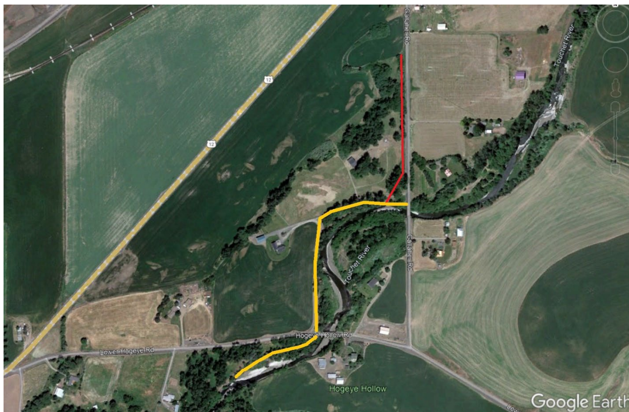
Figure 4. The proposed new levee (yellow line), including the return ditch (red line).
