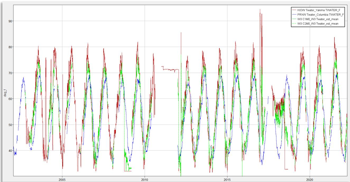
Figure 4-26. Timeseries of provisional hindcast estimates for mixing temperature at site W3 for WY 2004 to 2020.
