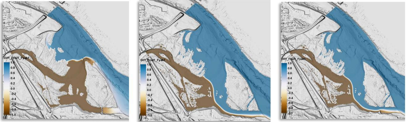
Figure 4-16. Simulations depicting mixing fractions of Columbia and Yakima River flows around Bateman Island on 28-June-2021. Left: Baseline (C0M0), Center: Full Causeway Removal (C1M0), Right: Partial North Causeway Removal (C2M0).
