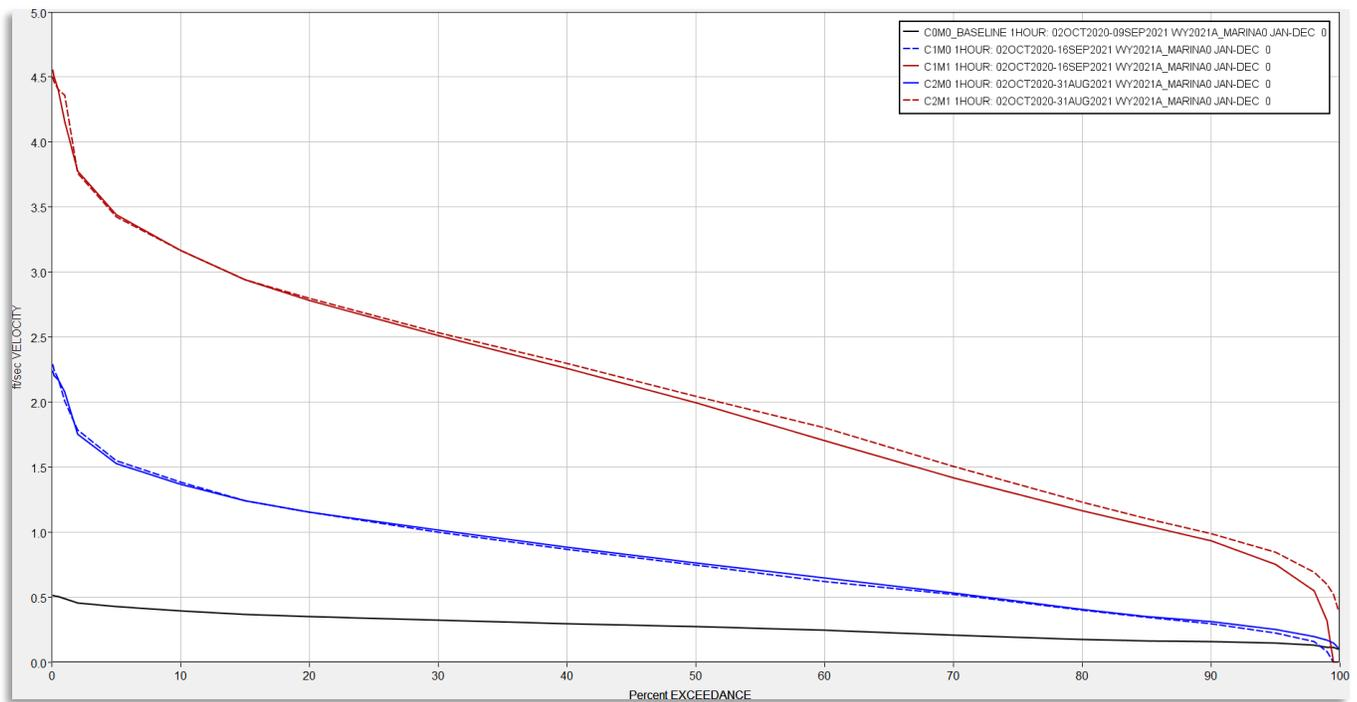
Figure 4-10. Exceedance duration of simulated velocity at the Marina causeway for Water Year 2021.
