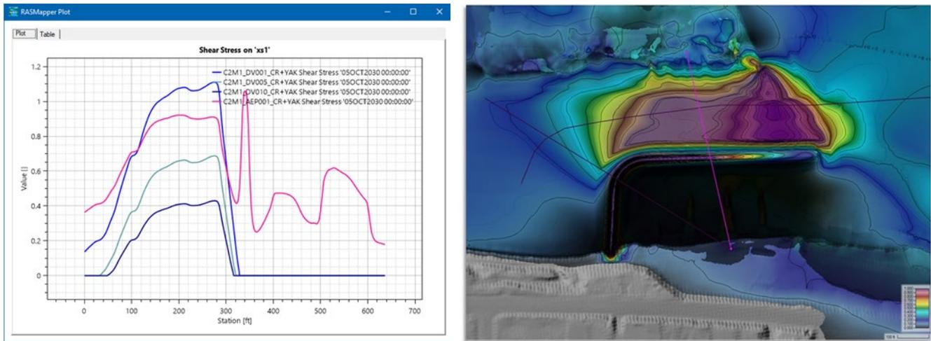
Figure 4-15. Shear Stress Cross-Section across M1: Levee Marina Barrier
