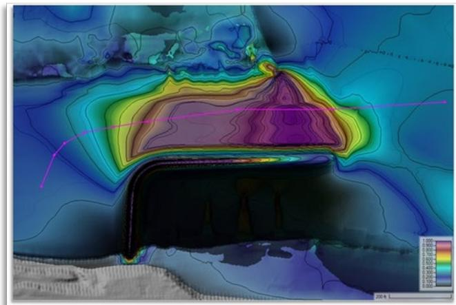
Figure 4-13. Shear Stress Profile along open causeway on North side of M1: Levee Marina Barrier
