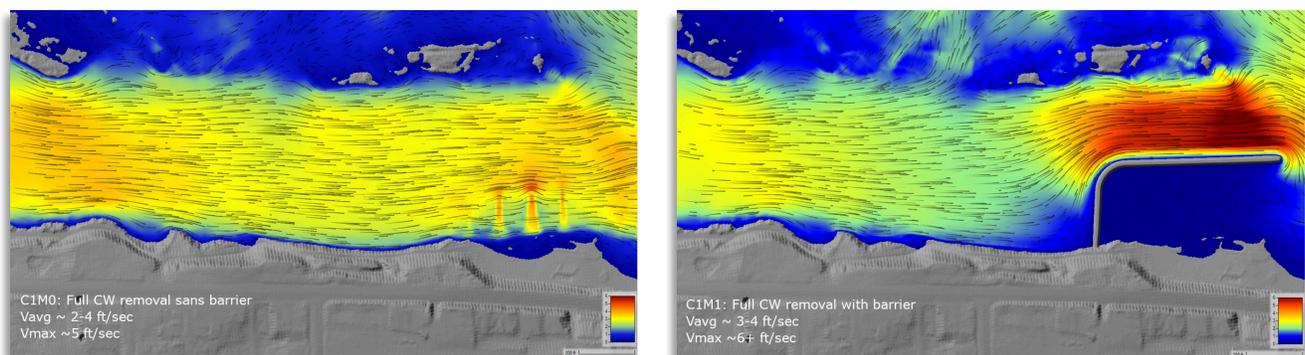
Figure 4-11. Simulated velocity for full causeway removal without (left) and with (right) marina barrier measure.
