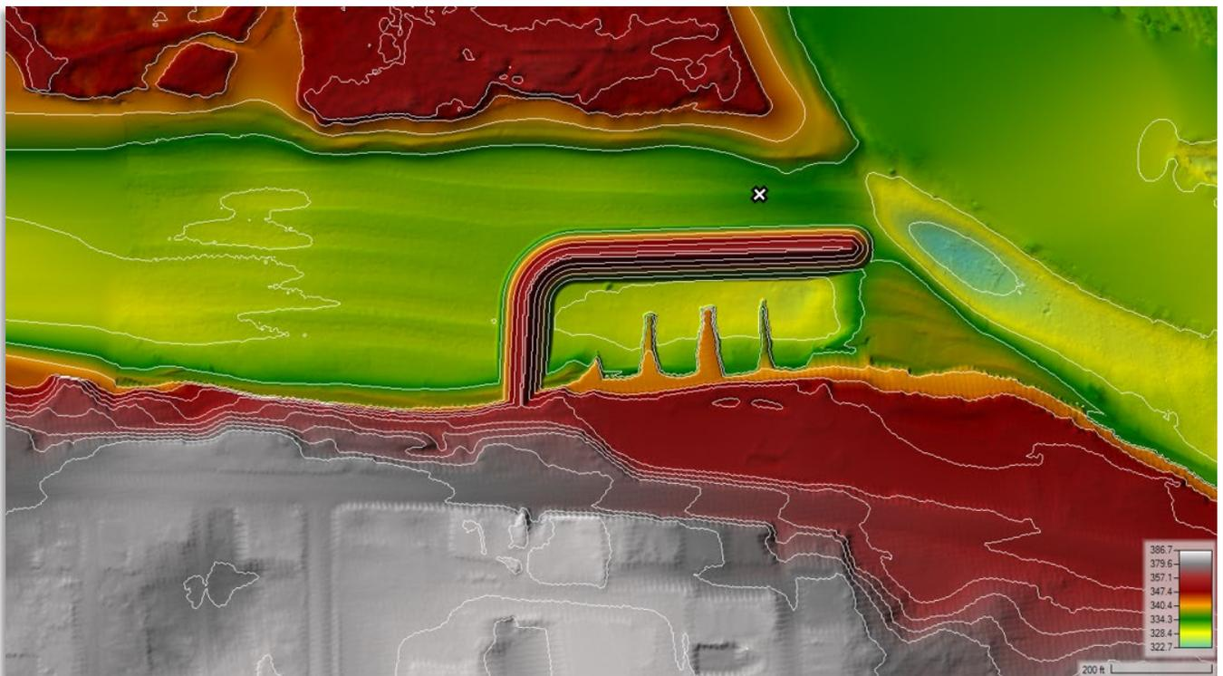
Figure 4-9. Layout for conceptual marina protection barrier levee M1 with velocity sampling location depicted.
