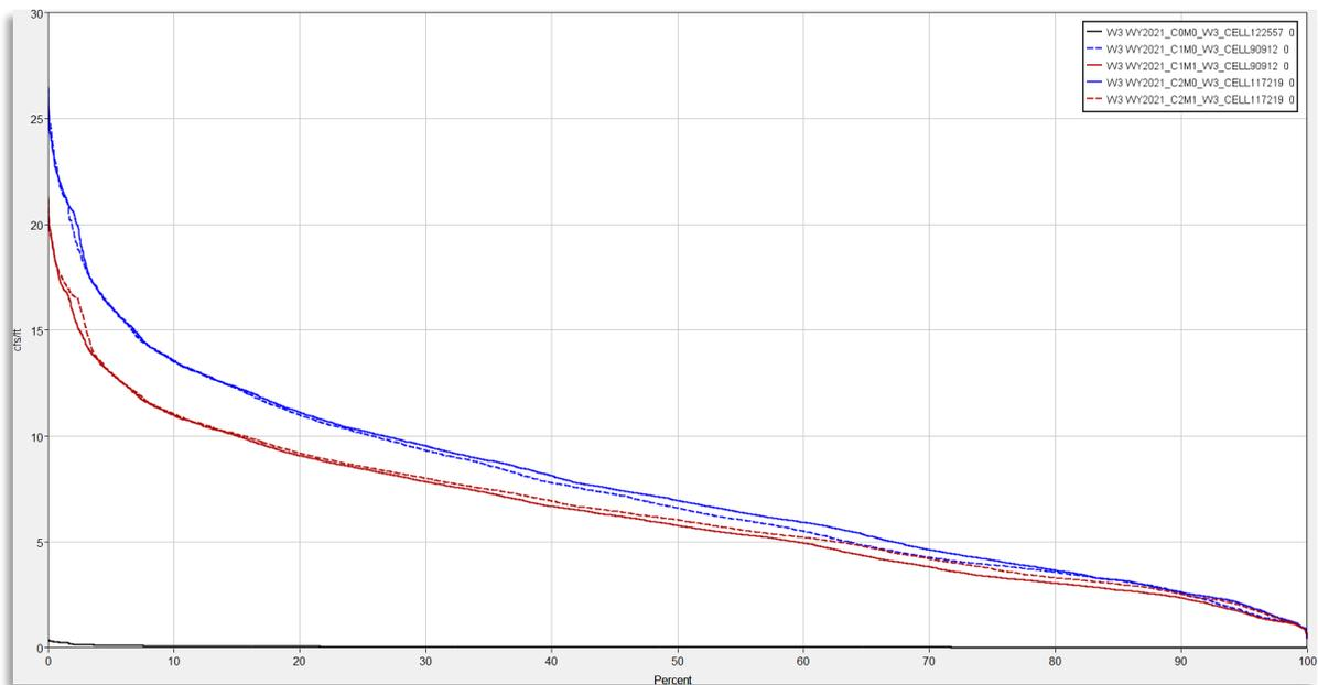
Figure 4-7. Exceedance duration of simulated unit discharge (cfs/foot) at site W3 for 15Apr through 15Nov - Water Year 2021. *Note the CO baseline of near-zero conveyance at the bottom of the plot.*
