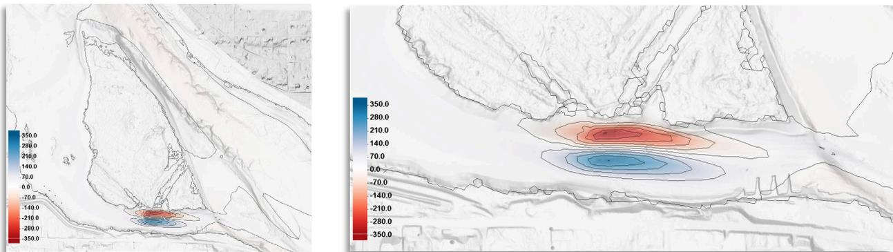
Figure 4-18. Difference in simulated cumulative unit volume (acre-feet per foot) between Full Causeway Removal (C1) and partial North Causeway Removal (C2) sans marina barrier over the March to September 2021 duration. Left: study area. Right: zoom to causeway corridor.
