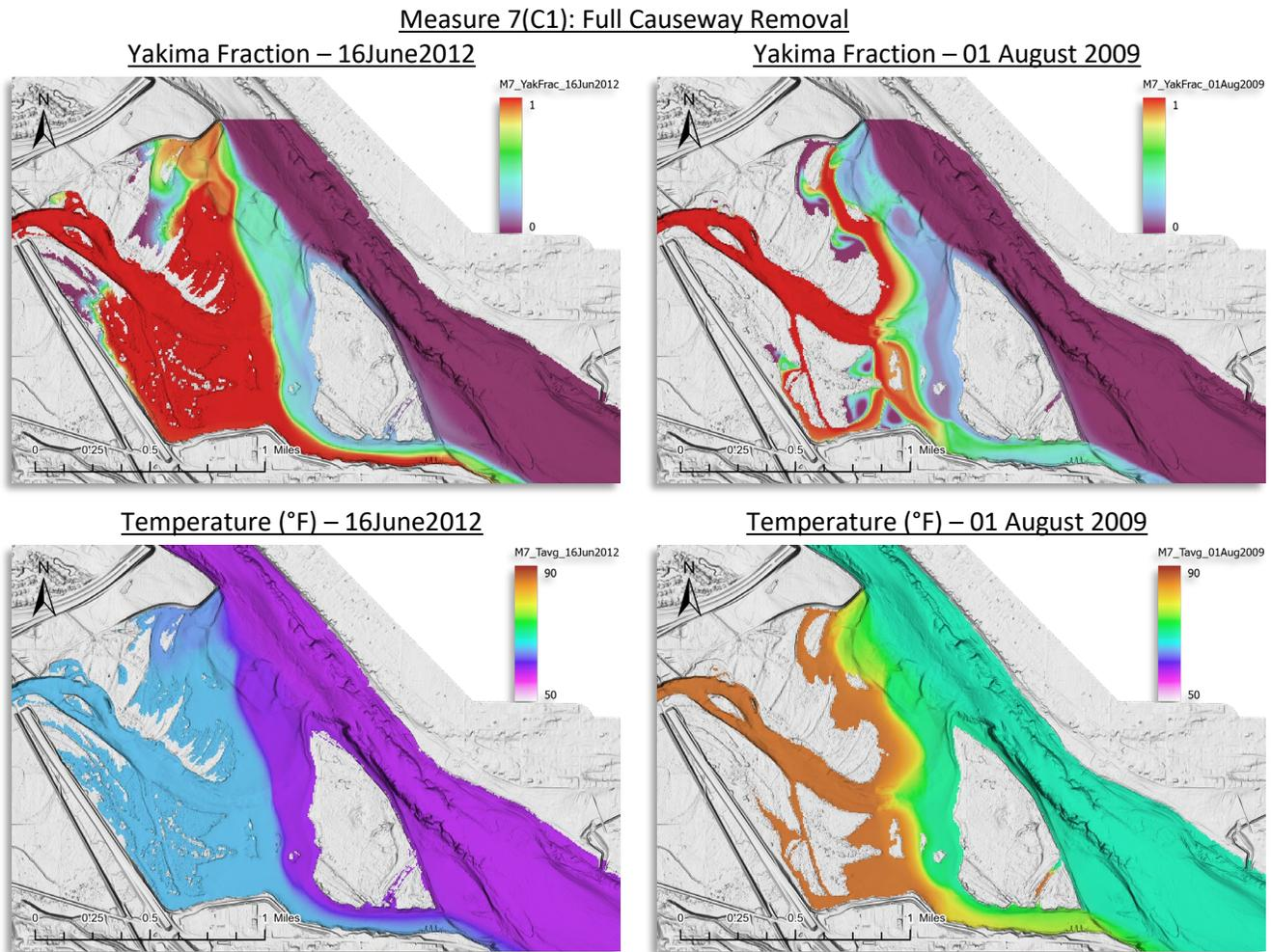
Figure 4-25. Measure7 (C1 – full causeway removal) simulation for late summer index conditions. (01Aug2009-High T, Low Q)
