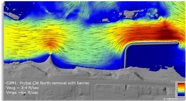
Figure 4-12. Simulated velocity for partial north causeway removal without (left) and with (right) marina levee barrier measure.
