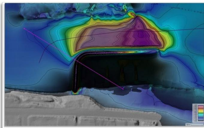
Figure 4-14. Shear Stress Cross-Section across upstream side of M1: Levee Marina Barrier
