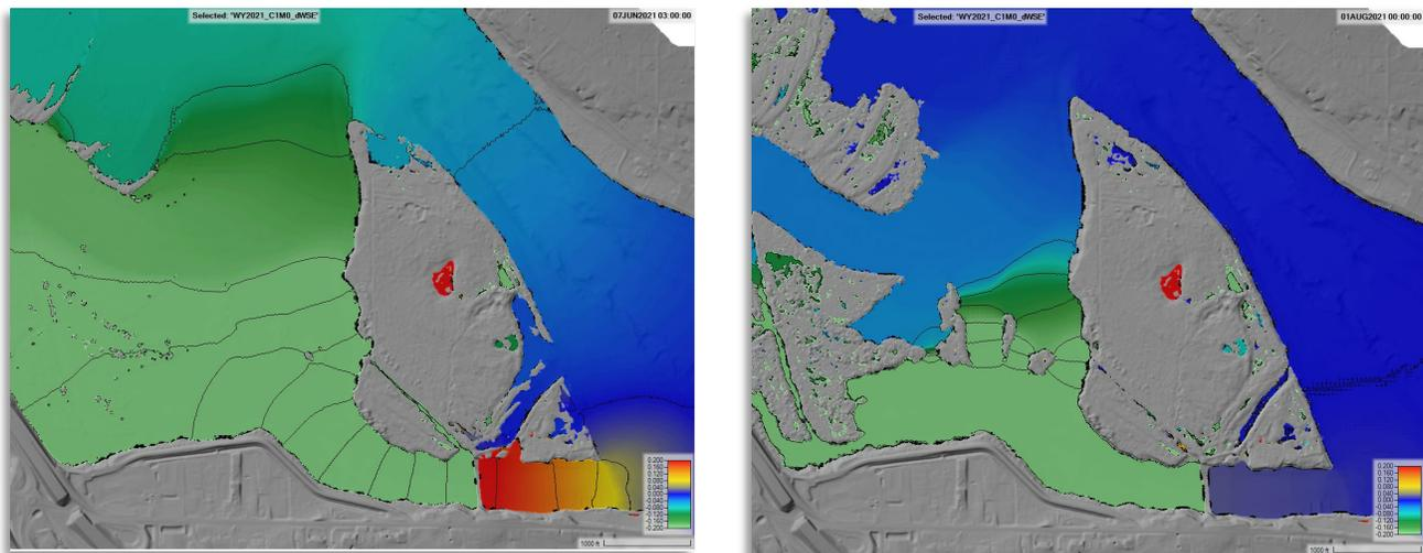
Figure 4-8. Comparison of simulated water surface elevations for full causeway removal (C1) minus baseline conditions (C0). Legend range spans from -0.2 feet (green) to 0.0 feet (blue) and +0.2 feet (red) with a 0.05 foot contour interval. Left: 07June2021. Right: 01August2021.
