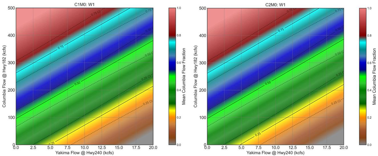
Figure 4-21. Provisional ratings with  $\alpha=0.05$  for Columbia River flow fraction at Site W1 near the north end of Bateman Island. Left: Full causeway removal (C1M0), Right: Partial north causeway removal (C2M0).
