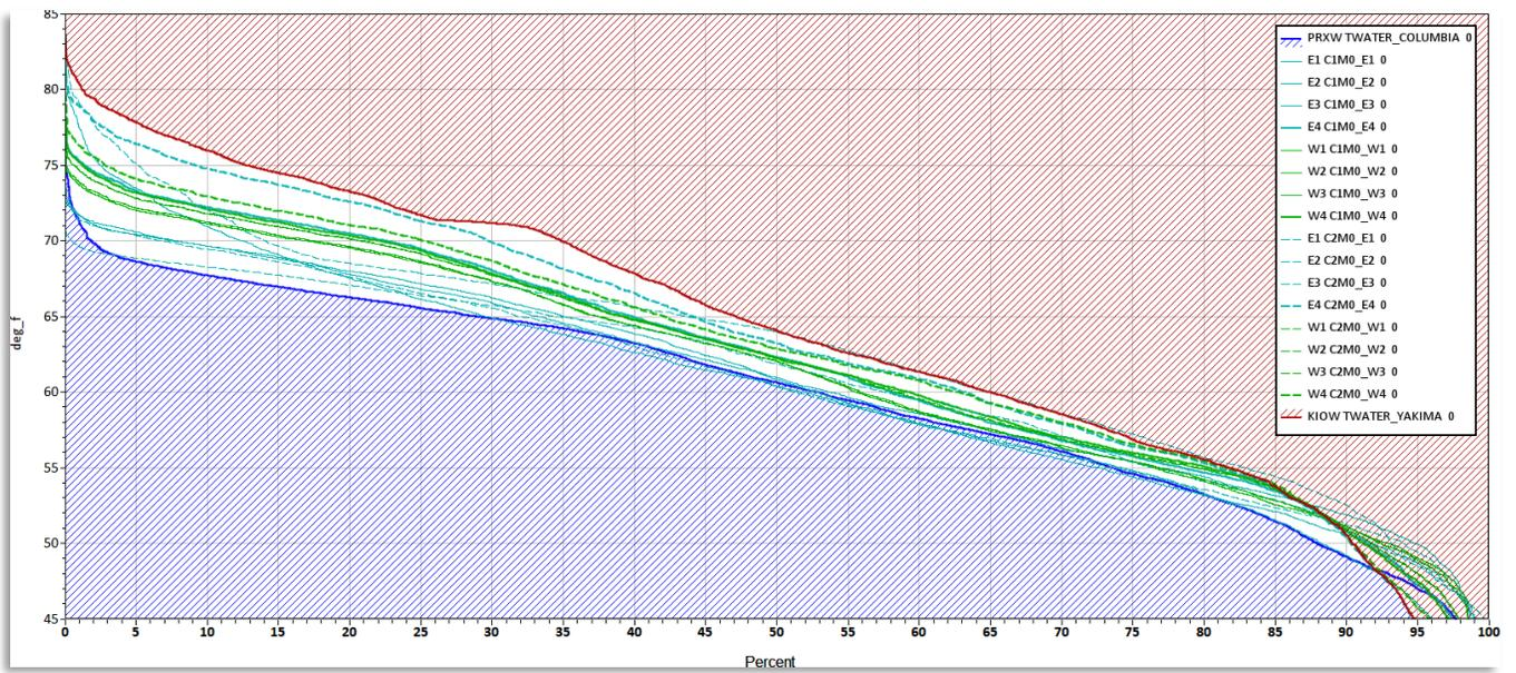
Figure 4-29. 15-April through 15-November Exceedance durations of provisional hindcast estimates for mixing temperature across sites W1-W4 and E1-E4 for Measure 7. *Potential for realized temperature benefits in the Yakima Delta fall within the unshaded plot area and varies by location.*
