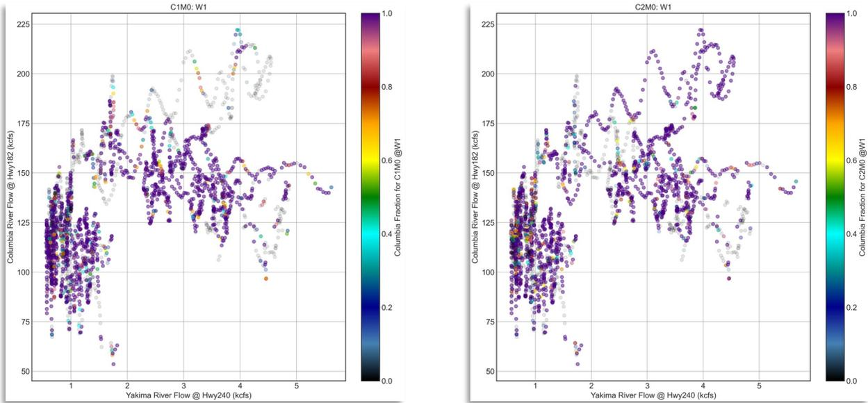
Figure 4-19. Simulated Columbia River flow fraction at Site W1 for WY2021. Left: Full causeway removal (C1M0), Right: Partial north causeway removal (C2M0)
