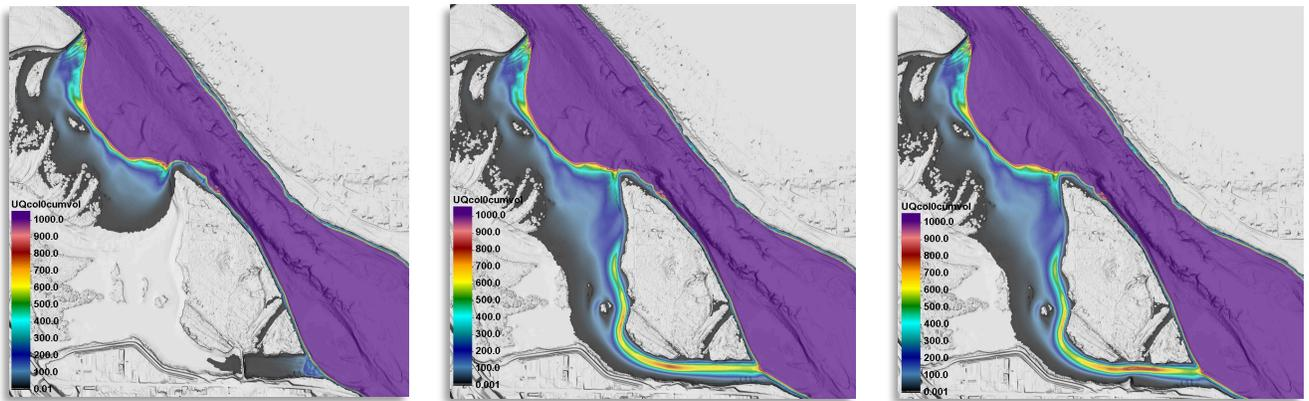
Figure 4-17. Simulated cumulative unit volume (acre-feet per foot) of Columbia River Water for March to September, 2021. Left: Baseline (C0M0), Center: Full Causeway Removal (C1M0), Right: Partial North Causeway Removal (C2M0). Note upper scale clipped to  $\geq 1$ kaf/ft to highlight Yakima delta patterns.
