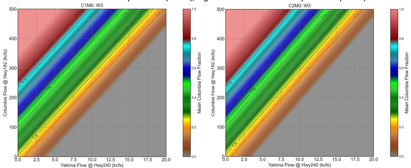
Figure 4-22. Provisional ratings with  $\alpha=0.05$  for Columbia River flow fraction at Site W3. Left: Full causeway removal (C1M0), Right: Partial north causeway removal (C2M0).
