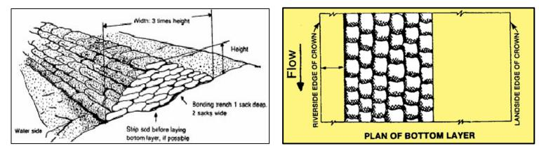
**Pyramid Placement Method** – The pyramid placement is used to increase the height of sandbag protection. Place the sandbags to form a pyramid by alternating header courses (bags placed crosswise) and stretcher courses (bags placed lengthwise). Stamp each bag in place, overlap sacks, maintain staggered joint placement, and tuck in any loose ends.
