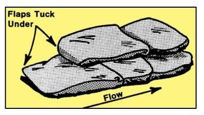
Stagger the joint connections when multiple layers are necessary. For unsupported layers over three (3) courses high, use the pyramid placement method (below).
