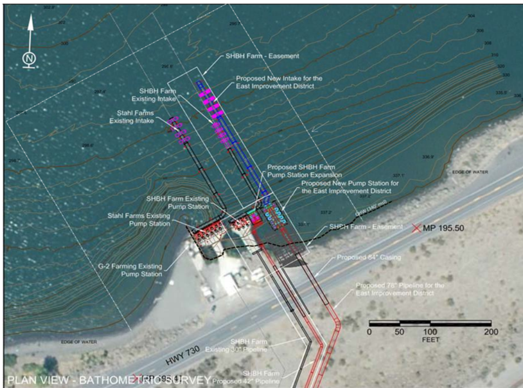
Figure 1: Project Site. Existing Pump Stations and Proposed New Intake Expansion.
