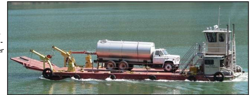
The Corps barge with fertilizer truck onboard. Nitrogen is applied from the tanker truck via pipes off the back of the barge and mixed into the water column by the prop wash.
