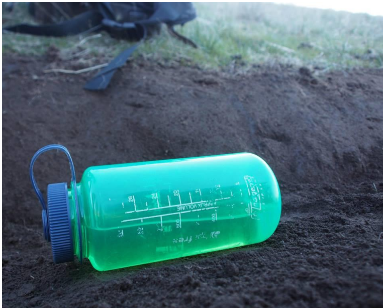
Figure 2 Using a water bottle check changes in running slope (along the tread)
