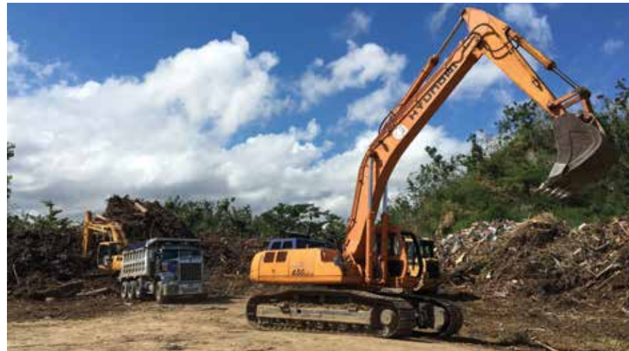
Left: An excavator repositions for operations unloading and loading trucks at the Trujillo Alta temporary disposal site. Temporary sites serve as municipal collection points for woody debris before it's reduced to mulch or transferred to another location for permanent deposition (mulch recycling site or landfill).
