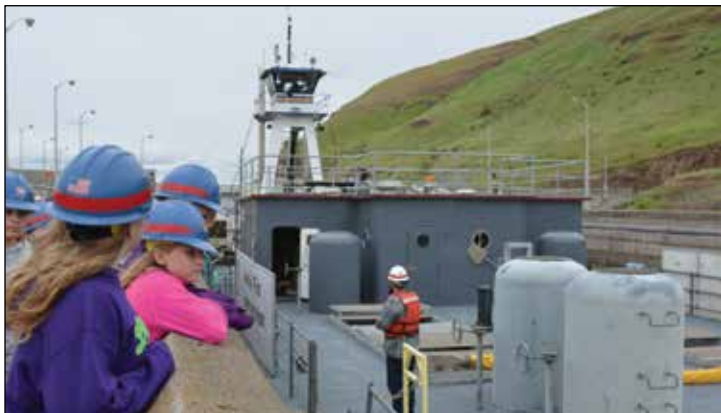
Students take notes as a tug prepares to push four loaded grain barges (approximately 800,000 bushels of red wheat) downriver after the navigation lock drained 46 million gallons of water and dropped 100 feet in less than 10 minutes.
