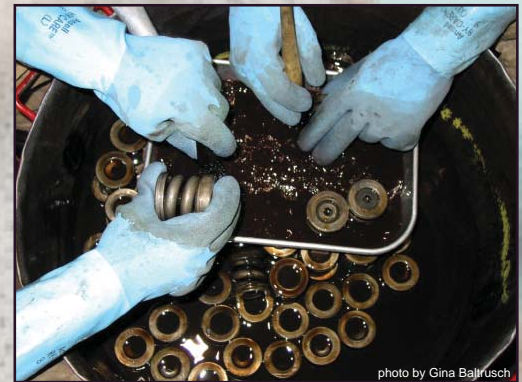
Lower Granite Lock and Dam crew members clean thrust bearings as part of turbine “unstack.”
