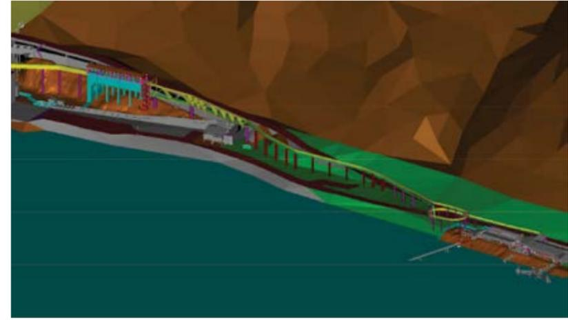
View of planned above-ground flume for the Lower Granite Lock and Dam Juvenile Fish Facility.
