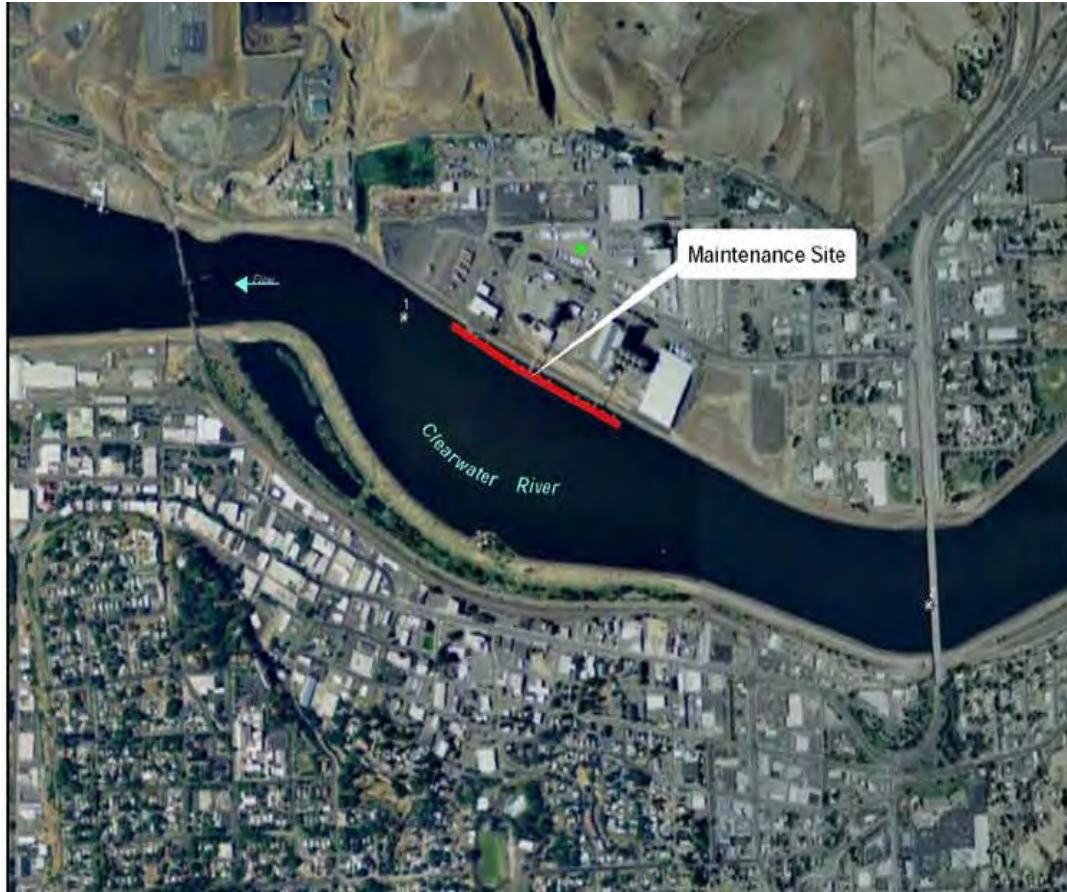
Figure 4. Dredging area at the Port of Lewiston, Idaho where the Corps will remove approximately 4,664 cy of material (Corps 2012).
