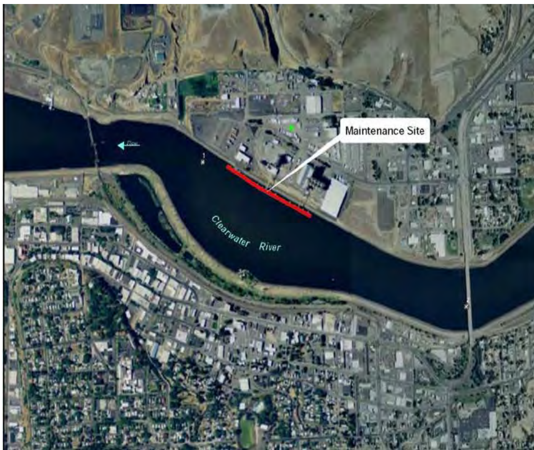
Figure 4. Dredging area at the Port of Lewiston, Idaho where the COE will remove approximately 4,664 cy of material (USACE 2012b).
