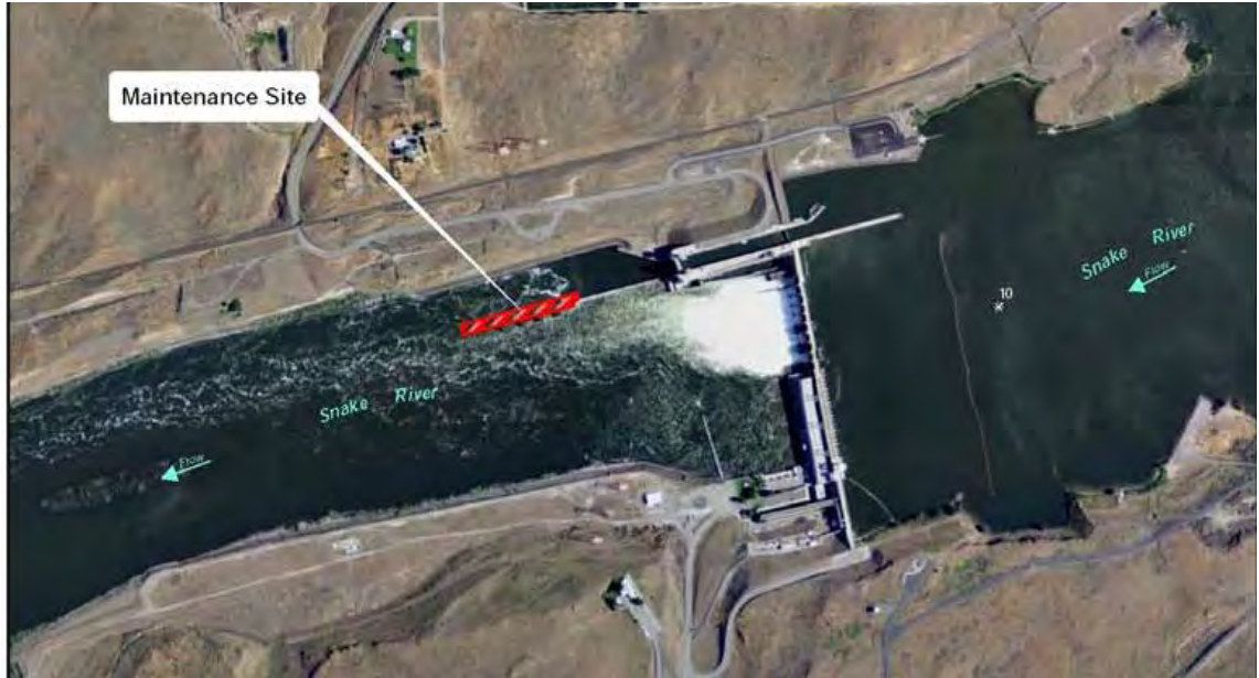
Figure 5. The Ice Harbor navigation lock approach where approximately 3,205 cy will be dredged and barged upriver to the Knoxway Canyon site.
