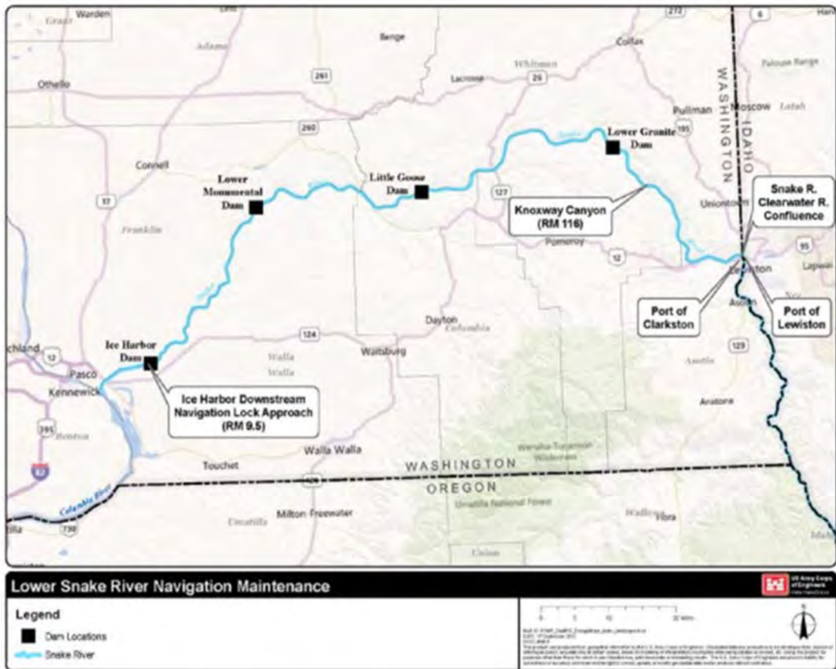
Figure 1. The Federal navigation channel in the Lower Snake River from the confluence with the Columbia River to the confluence with the Clearwater River at Clarkston, Washington. The four dredging locations are the navigation lock approach at Ice Harbor Dam, the Federal navigation channel at the confluence of the Snake and Clearwater Rivers, and the Ports of Lewiston and Clarkston. Dredged material will be used as fill at the Knoxway Canyon bench site to create shallow water habitat (Corps 2012b).
