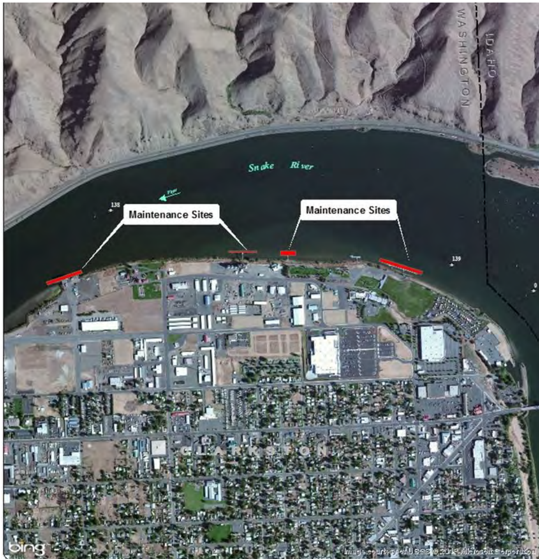
Figure 3. Port of Clarkston berthing area where the Corp will dredge approximately 14,143 cy of material (USACE 2012b).
