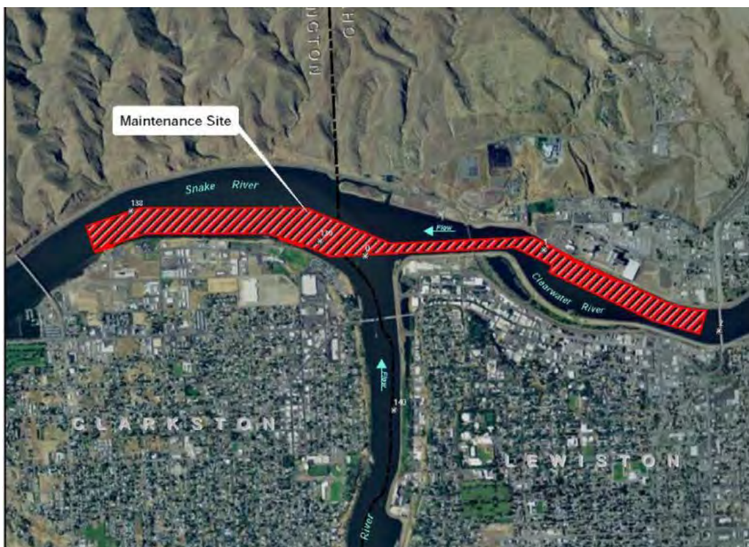
Figure 2. Confluence of the Snake and Clearwater Rivers with the Federal navigation channel dredging area identified. The Clearwater River enters from the east, the Snake River flows in from the south and continues downstream to the west. The Lower Granite Dam is approximately 39 miles downstream (west). The Corps will dredge approximately 458,472 cy of material and barge it downstream to the Knoxway Bench site (Photo courtesy Corps BA 2012).
